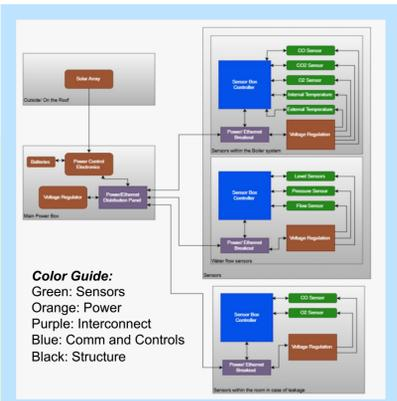
System block diagram for sensors within the boiler system
