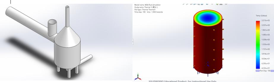
SolidWorks simulation for the heating process
